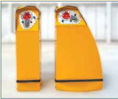
R66 Aux Fuel Tanks
